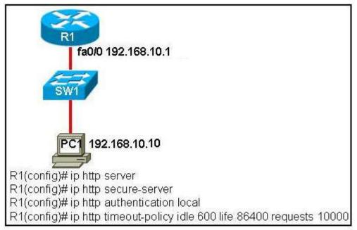
Refer to the exhibit. Security Device Manager (SDM) is installed on router R1. What is the result of opening a web browser on PC1 and entering the URL https://192.168.10.1?
